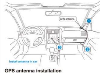
1.Clean adhesion area with oil-soluble detergent, and fix GPS antenna with adhesive tape tight.
