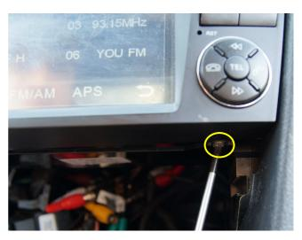
Then the radio can be removed up front. In doing so slightly tilt it. Then disconnect the connectors on the back. (If not happened until now, please turn the ignition off before.)
