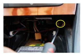
Then the control panel can be removed up front. In doing so slightly tilt the control panel. Then disconnect the connector on the back.
