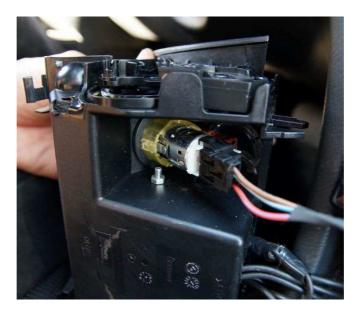
Next we remove the control panel. For this you must loosen two screws underneath the control panel with the Torx screwdriver.
