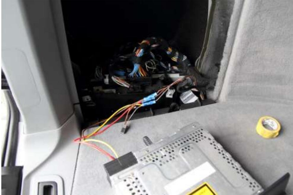
25. Using 16 gauge spade connectors, connect the wires to the CD player in the following order: Red to pin 15, brown to pin 12, and yellow to pin 9. You can see the pin numbering if you look closely. Make sure the spades on the pins are tight and don't move around.
