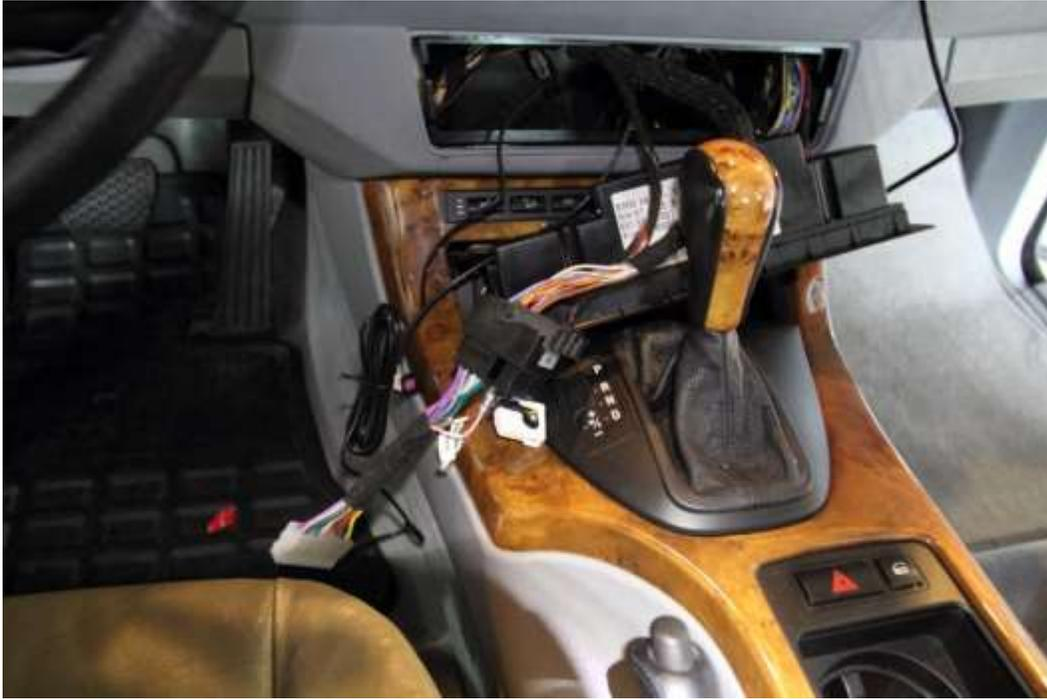
29. Plug in the wiring harness, camera, antenna and any other cabling into the back of the Avant-2 and slide into place. Having the AC controls out of place helps give space for placement and cable management. **The deck should fit snugly, no additional screws needed to secure it.**
