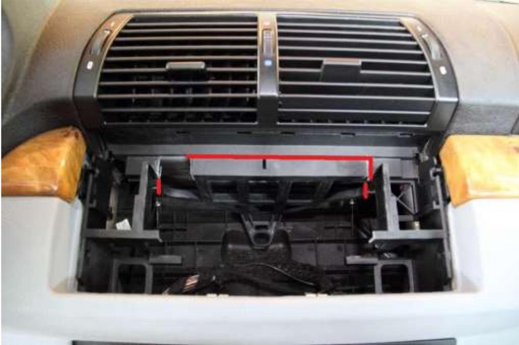
11. **CHECK FIT** for the deck! Again note, do not remove the middle bar. If the deck will not smoothly slide into place, and is too tall we will need to remove more framing. The deck should fit **VERY SNUGLY**, and not move at all when in place.
