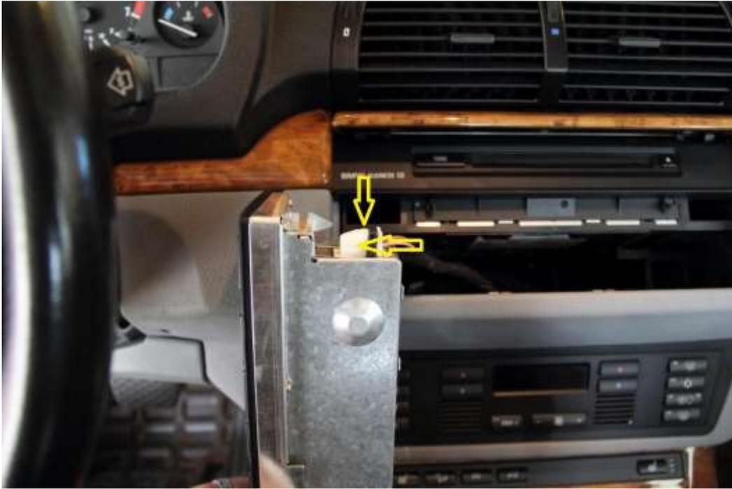
5. Remove the two indicated screws and gently slide the CD player out of the dash.
