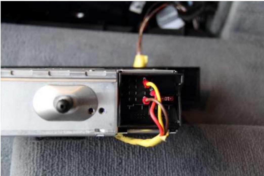
26. Secure CD player in the compartment and close it back up. Make sure your spade connections and wires are secure. I used a large Velcro pad to hold the player in the compartment.
