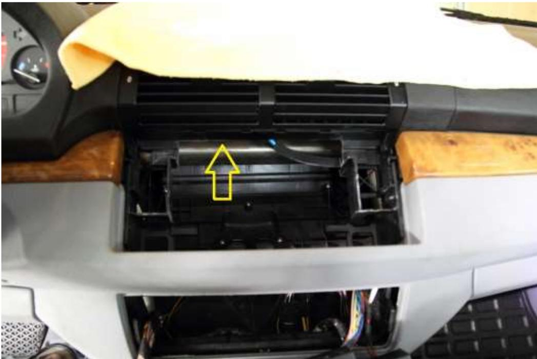
28. Connect the provided wiring harness adaptor, camera, USB, iPod and any other accessory cabling as desired.
