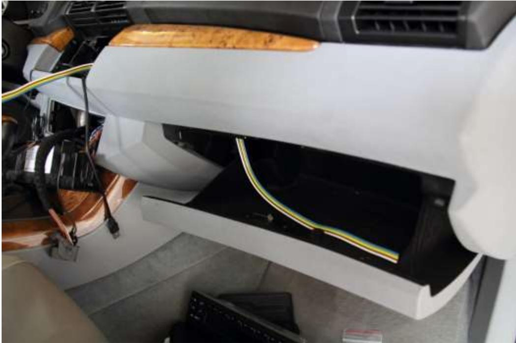
21. Cut off the white plug for the OEM mid section, with at least 3" of wire from the plug. Strip and connect 5 wire bundle to mid wires using butt connectors. (or your preferred method)
