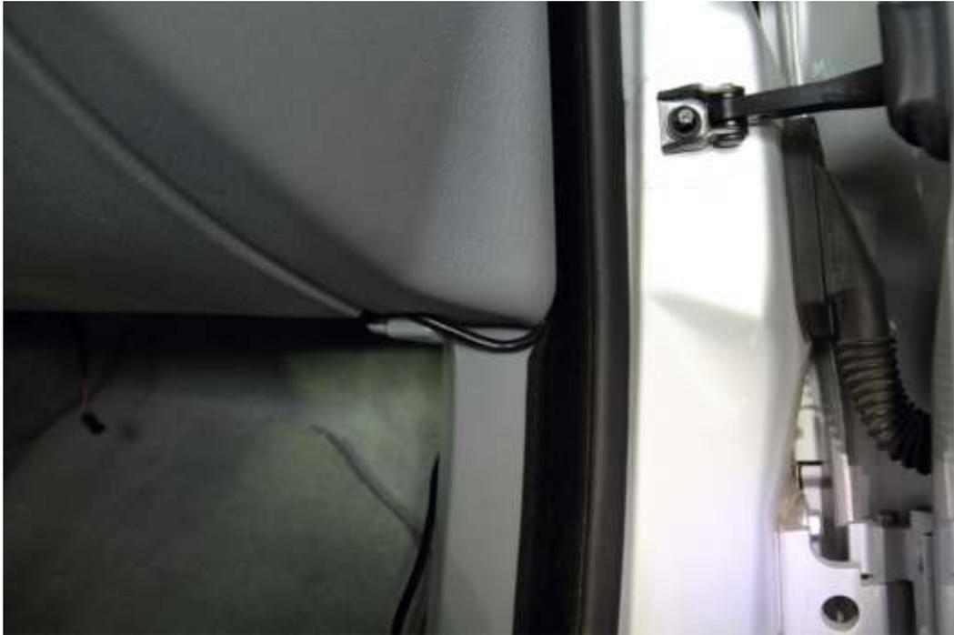
19. Continue the cable run behind the glove box and up into the dash. You can remove the small panel below to help give space to route the cable. Replace panel once done.
