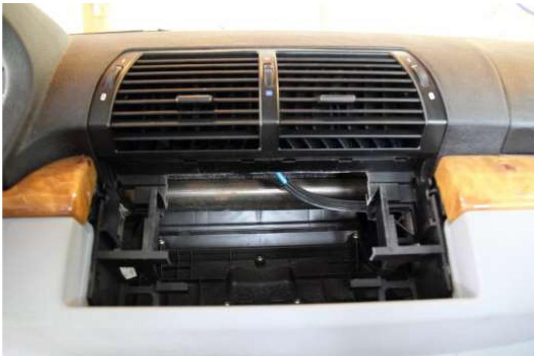
14. I wanted the deck to sit a little deeper into the dash to be more flush. I removed the front edges marked in red to give more depth. Note the AC controls are removed below to give more room to work. It pushes out from behind easily with your fingers.
