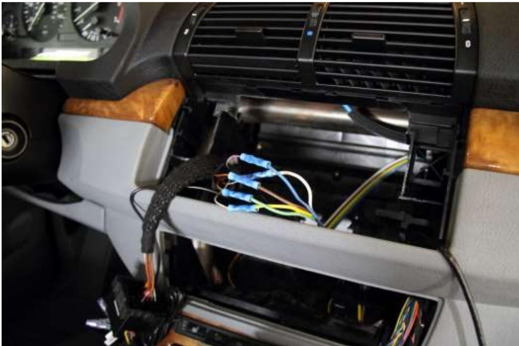
22. Connect white plug to wire bundle in the glove box, make sure to wires are matched properly at either end. Bundle colors don't matter as long as they match at both ends. Red to red, brown to brown, yellow to yellow etc. Plug the mid section back in and secure in the glove box. I used a Velcro pad on the bottom to ensure it wouldn't move around. You obviously lose some space.
