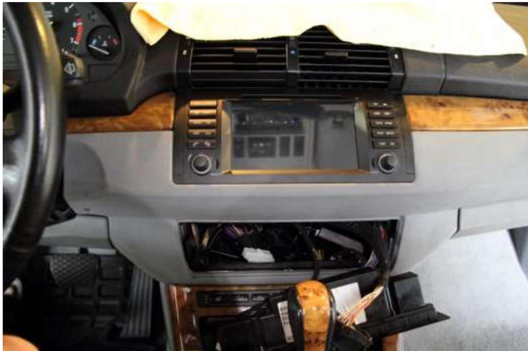
30. With everything connected, turn on the ignition and power up the deck (**IF DSP, mid section in the glove box turned ON**). Before closing everything up, make sure everything works. Check GPS reception, radio strength, and wireless connectivity and so on. Also, it is a good idea to check if there is a newer OS build for your deck as AvinUSA continues to make build improvements over time.
