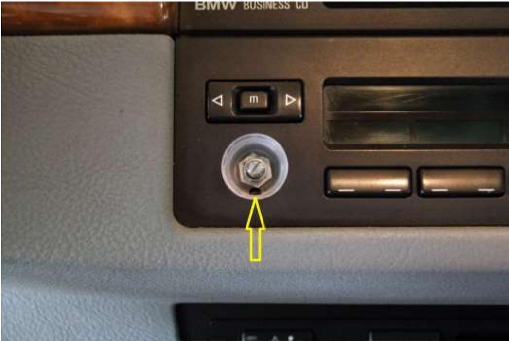
3. Use the T-10 in the hole to gently pry out the mid section, or gently grip the volume knob peg with pliers and pull out of the dash.
