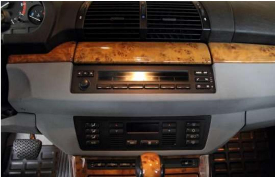
2. Use T-10 torx into the small hole, and turn a ¼ turn to the left to unlock the mid section.
