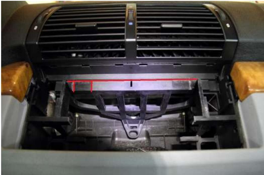
10. Score the top line heavily with a utility knife, and then break out the small square using pliers. It should break off cleanly. Then use hack saw blade or dremel and cut the remaining top line carefully, and also cut free the two curved arms of the frame to free it completely.
