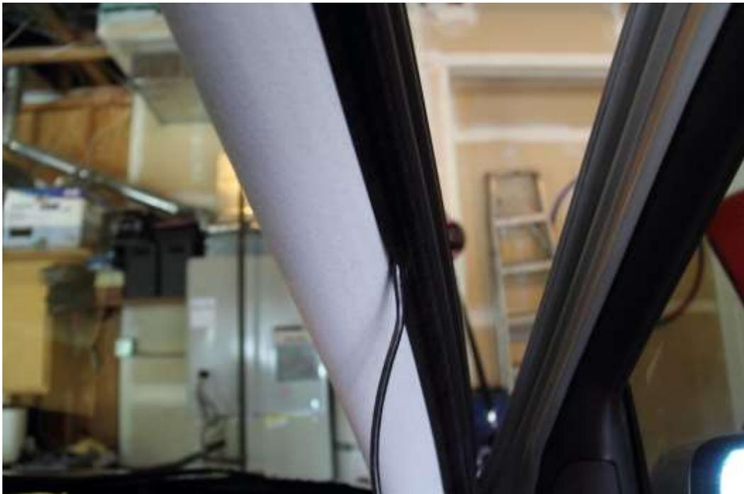
18. Route cable down to the glove box hinge, running above the hinge and behind the panel. Use the plastic trim tool to help guide the wire behind the weather stripping.
