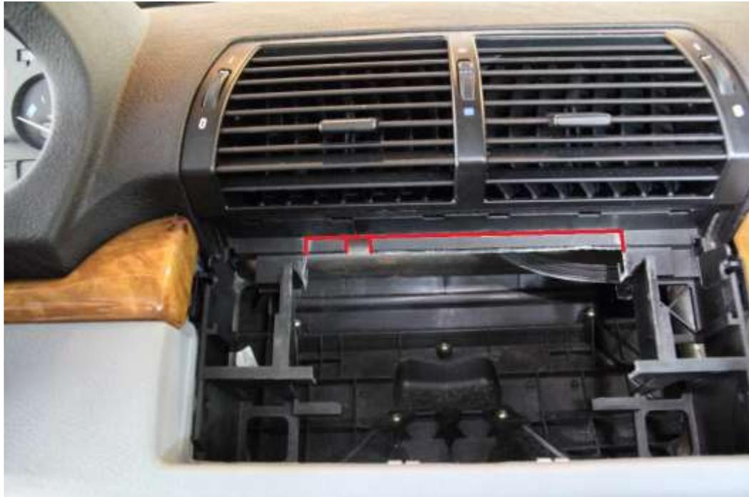
13. **CHECK FITMENT of the deck.** For me at this stage, the deck easily slides into place and fills the space properly. Also check deck depth into the dash, as mine needed to be deeper to be flush.
