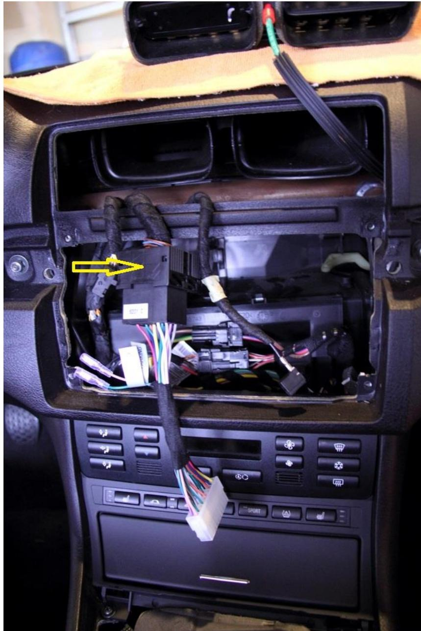
19. Connect the wiring harness to the back of the Avant-2, along with antenna wire and any other accessories. I attached the (1) 3G USB modem, (2) Canbus interface and (3) Ext. line to the top of the deck using provided Velcro pad. The (4) GPS antenna is installed on the brace below the vent ducts as it is magnetic and stays there perfectly.
