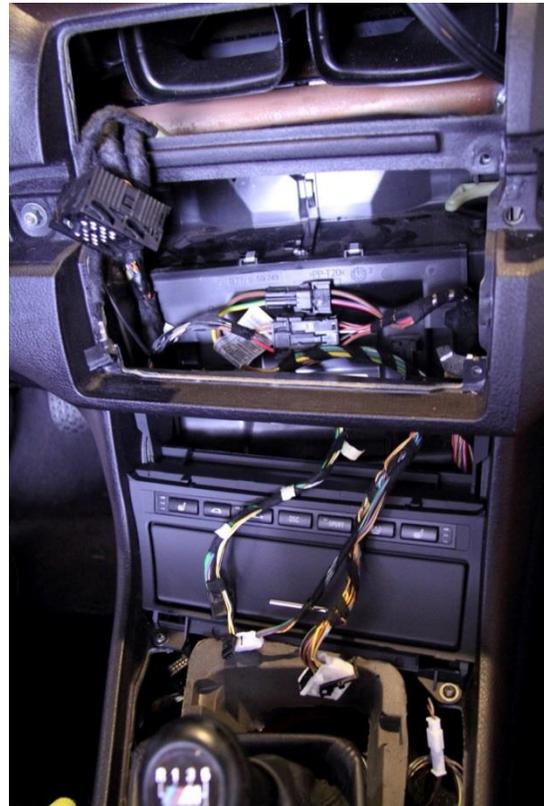
17. Connect the HVAC controls to the module and gently snap into the opening, guiding cables at the back from the top if needed. Reverse the order to reinstall the gear shift surround and window controls. You won't need access to that area moving forward.
