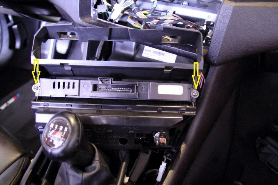
15. The lighter/power outlet socket will need to be removed from the old frame and installed into the new frame. The socket is secured in place by two plastic tabs and once unlocked, pushes out the front.
