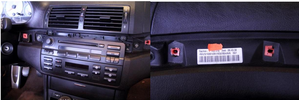
4. Use a pair of needle nose pliers to grip and then remove the trim clips. Turn the clip to a vertical orientation to remove and pull out. Insert the new clip vertically and then turn horizontal to lock into place. The blade of the pliers works well to turn back into place.
