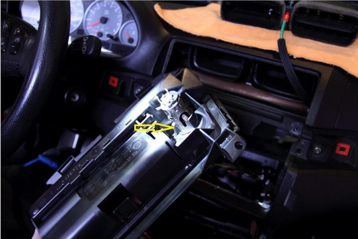
16. Install the new frame, plug the socket and buttons back in and gently install into place. Secure the frame using the same four screws, and pull HVAC cabling down into the new frame.
